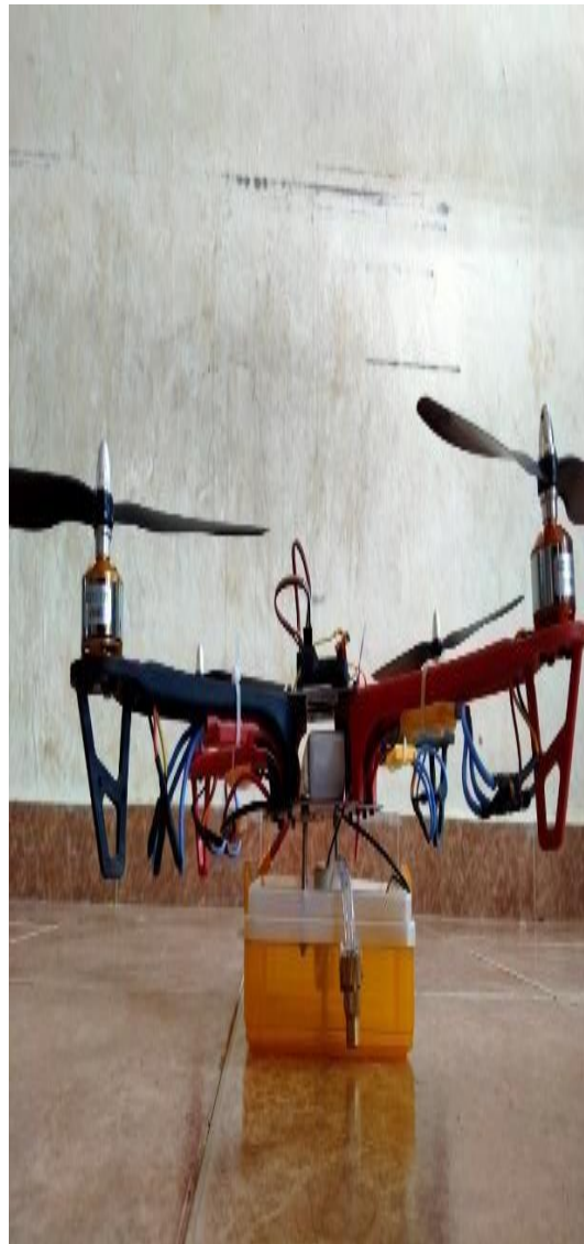
Fig. 3 Quadcopter with spraying system
