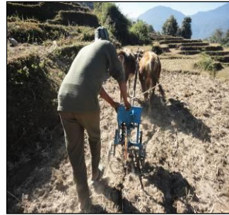
Fig. 2. Single row seed drill for mustard
