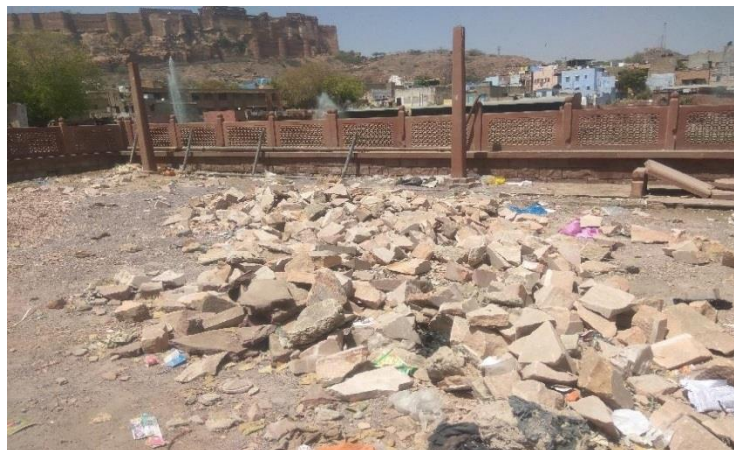
Figure 3. Sandstone renovation waste at Gulab Sagar, Jodhpur
